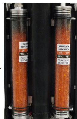
Silica gel desiccants in the fixture arm
