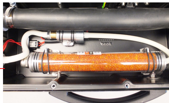
Silica gel desiccant in the fixture base
