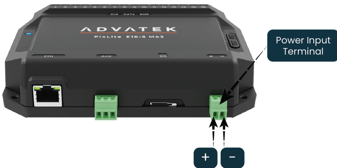
Figure 6: Location of Power Input
