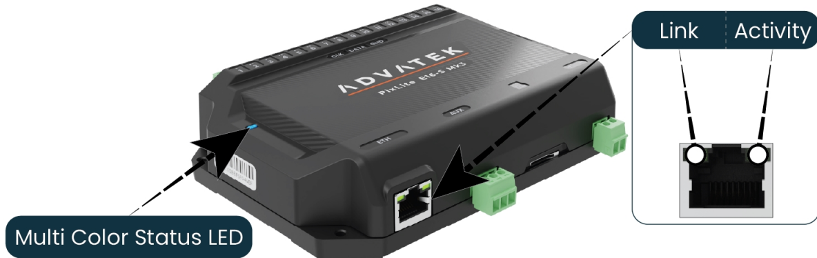
Figure 17: Location of LEDs
