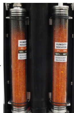
Silica gel desiccants in the fixture arm
