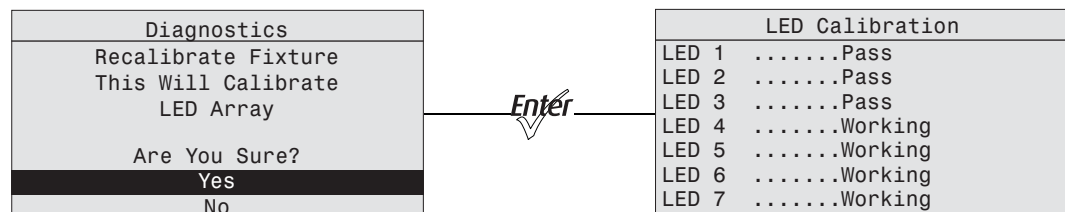
Figure-4.36 LED Calibration screen with calibration in process
