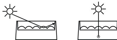
Figure 2: Risk of sunlight damage
